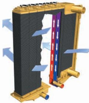
**Next Generation Modular Radiator (NGMR).** Improves cooling capabilities by using a parallel flow system with six cores. Serviceability is improved with NGMR since there is no top tank to remove.
