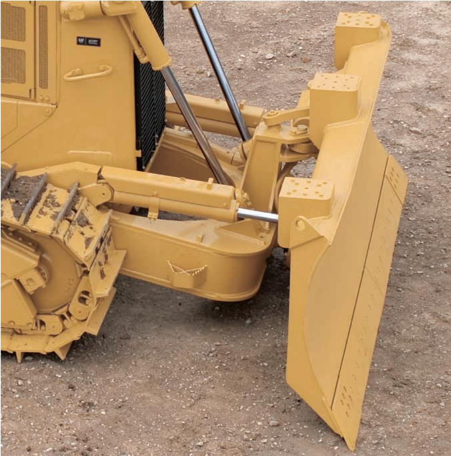
**Cat® Blades.** All blades feature a strong box-section design that resists twisting and cracking. Blades are made of Cat DH-2™ steel that has high tensile strength and stands up to the most severe applications. Heavy moldboard construction and hardened bolt-on cutting edges and end bits add strength and durability.
