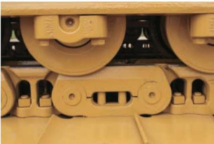
**Master Link.** A unique feature of the System One Undercarriage is that, unlike traditional undercarriage, a master style link is not required. This improves track reliability and durability. The unique straight link design allows the track to be taken apart at any joint by using the proper Caterpillar tooling to press the link on or off.
