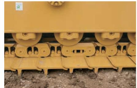
**Roller Design.** The SystemOne™ roller has a taller flange to improve track guiding, especially in side-sloping applications. Advanced features and reduced piece parts enhance the rollers which help eliminate any flexing in the collars and avoid oil loss. The roller is maintenance-free and serviced as a group only. To achieve total balanced wear, carrier rollers with increased wear life are also used.
