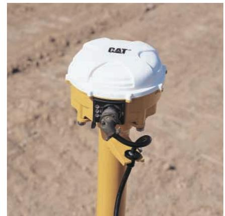
**AccuGrade GPS.** AccuGrade GPS computes the positioning information on the machine, compares the position of the blade relative to the design plan and delivers that information to the operator via an in-cab display.
