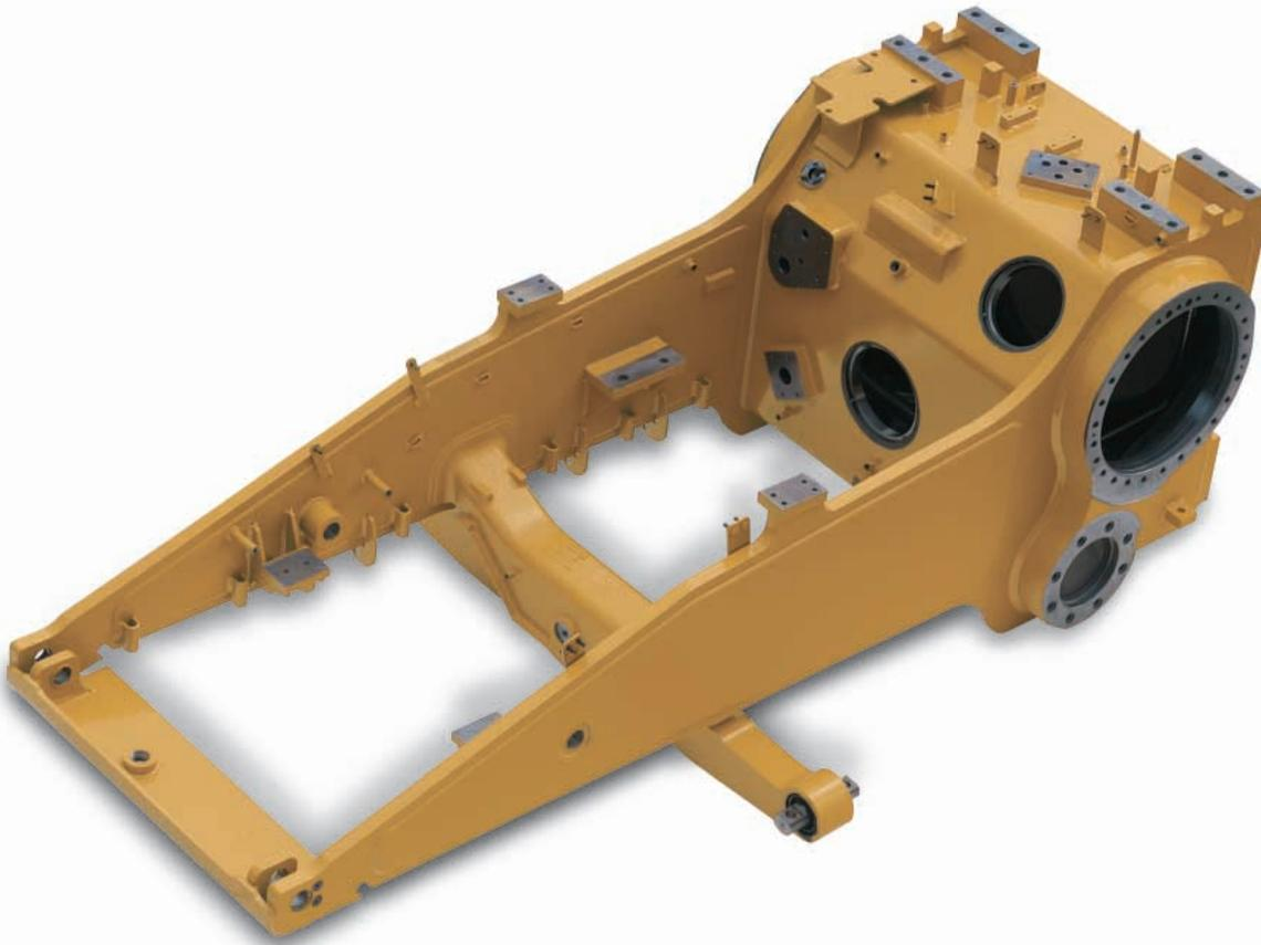
**Frame and Castings.** The D6T frame is built to absorb high impact shock loads and twisting forces. The frame has a reinforced saddle and a welded front cross-member that add strength to the frame to better handle lateral and twisting forces. Steel castings augment the strength of the main case.
