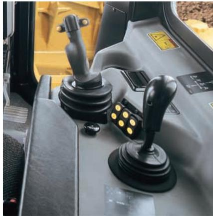
**Work Tool Lock-Out Switch.** Redesigned from a mechanical rotary switch to an electronic rocker switch, the work tool lock-out valve prevents inadvertent operation of the hydraulic work tool attachments.
